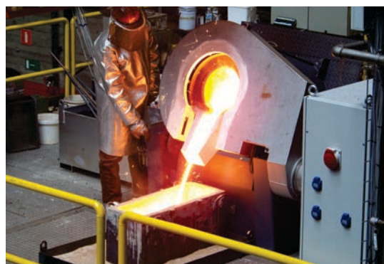
Byproducts processing facilities – Smelting furnaces 350 kg induction furnace dedicated to the recycling of solid residues in metallic bath
